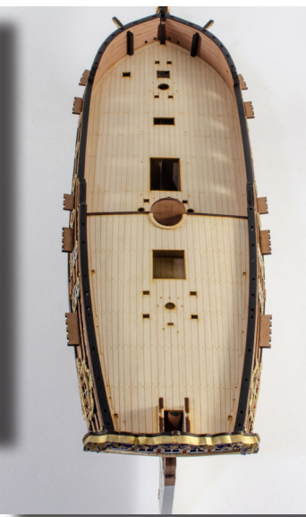
146. Cut the two sets of Channel Edging Strips (209, 210, 211, 212) from the 1mm wood sheet, and fit to the edges of the channels you just installed. You will need to slightly curve the fore channel parts in hot water. Glue these to the corresponding channels.
