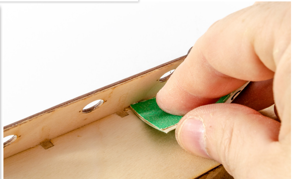
88. The temporary beams can now be twisted and broken off the hull, followed by the MDF bulkhead tabs above the decks. A knife and sandpaper were used to make these flush to the deck. Any glue remnants were also removed from the inner bulwarks.
