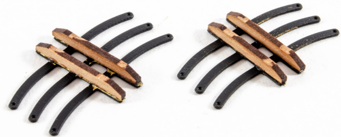
225. Take the Fore Topmast Trestletrees (175) and the Main Topmast Trestletrees (176) from the 1mm wood sheet. Also cut the Fore Topmast Crosstrees (105) and the Main Topmast Crosstrees from the 0.6mm photo-etch sheet. Glue the corresponding parts together as seen here and on plan sheets 8 & 9. Drill a 0.6mm hole through the timber, from the holes in the PE.
