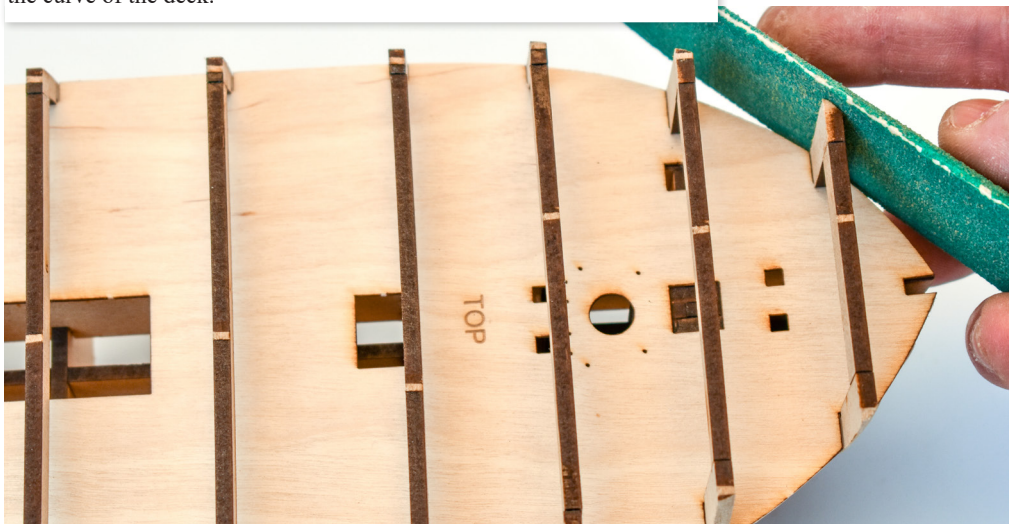
61. It's important that you sand the bulkhead edges so that they match the curve of the deck.
