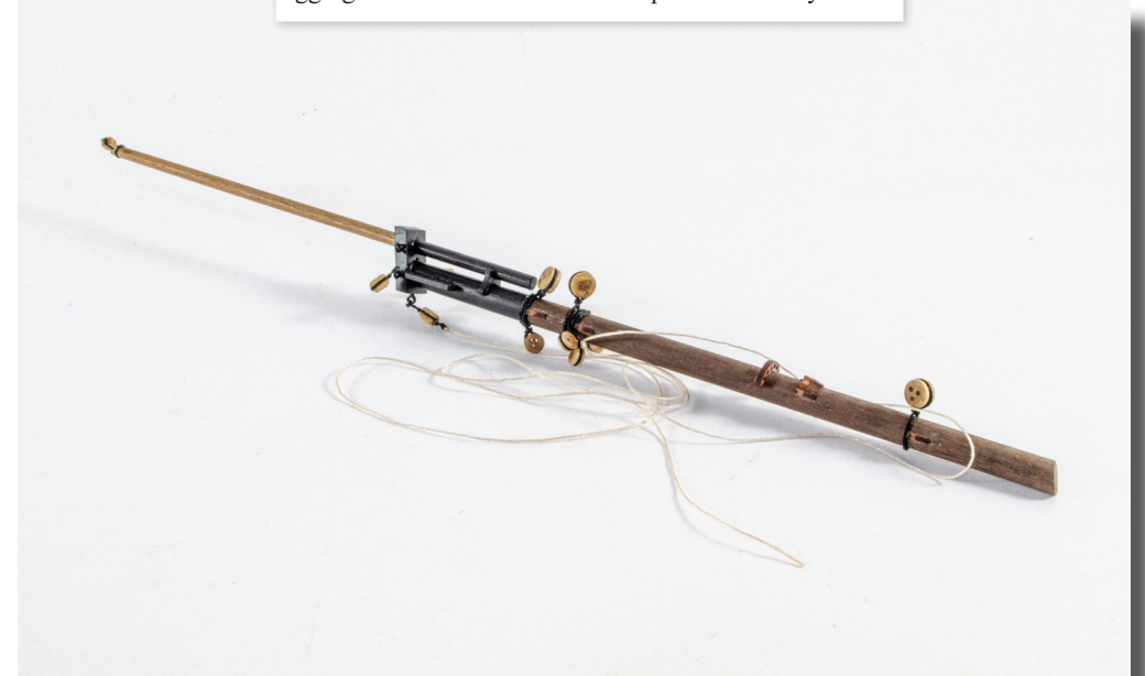
230. Build the bowsprit as shown on plan sheet 10. Fit it out with eyelets and paint black as shown. Finally, fit the rigging blocks and varnish the completed assembly.
