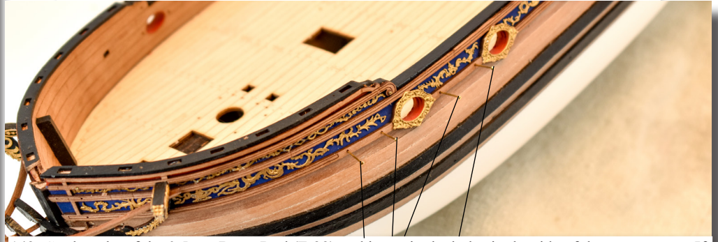
143. Cut lengths of the 0.5mm Brass Rod (F-39) and insert in the holes in the side of the pear pattern. If you wish, you can drill these holes a little deeper into the bulwarks but be careful not to break out of the other side. Glue the wire and cut so a few millimetres are sticking out.
