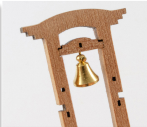
184. Cut the brass pin shorter and glue the bell into the head stock. Now glue the head stock into the bell standard.
