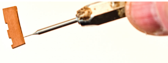
144. Using the plans, place the correct channel at each position and mark a point to drill the edge of the channel.
