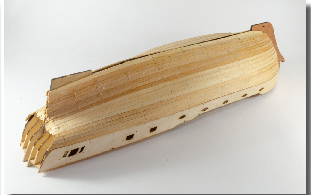
73. Your planked hull should look something like this, as shown in these four photographs. All that matters at this stage is that you have a good surface onto which you will lay the next layer of planks.
