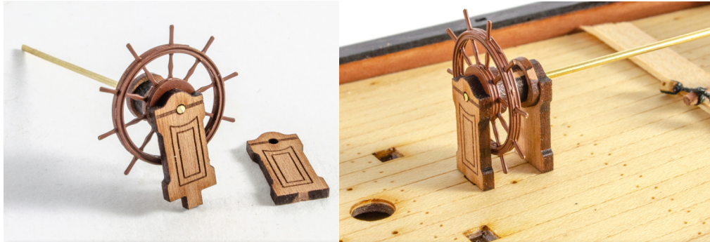
158. Glue the for and aft Ship's Wheel Standards onto the wheel assembly. You can temporarily sit this on the deck to ensure the aft part is level with the deck. When dry, cut the brass rod flush with the side of the assembly.
