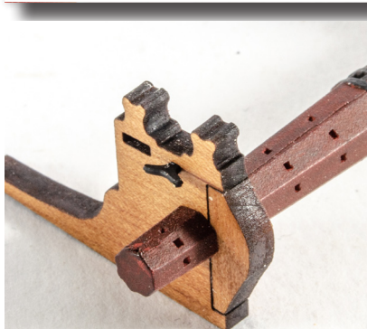
191. Sit the winch drum in the cut-out in the Windlass bitts and glue the Front Pattern into place. Don't glue the actual winch drum. Fit the bitts to both sides of winch drum.
