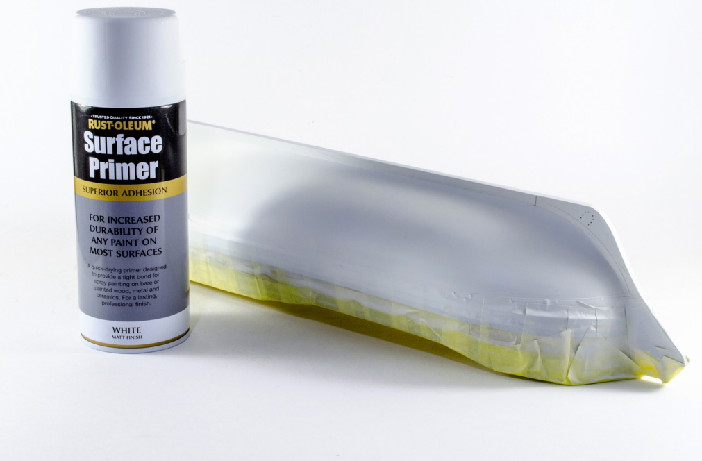
108. The lower hull is now sprayed with white primer and built up in thin coats. If you see any gaps, they can be filled and then sanded back. For the prototype, we used acrylic thinner, but heavily diluted with water and then brushed on.
