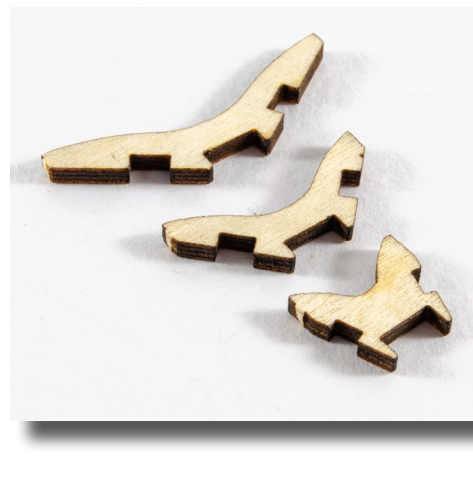
122. Cut the Bow 'V' Frames (33, 34, 35) from the 2mm ply sheet, and file them to shape as shown here. The filing will angle the slots on one side, and also bevel the outer corners. Glue these into place on the prow, as shown. Paint these parts black apart from the surfaces where the rails will fit.
