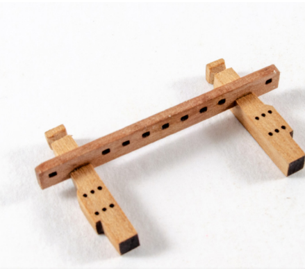
173. Cut the Main Mast Bitts Aft Belaying Rail (150) from the 1mm wood sheet, and also the two Main Mast Bitts - Aft (57) from the 3mm wood sheet. Remove the char and assemble as shown. You can now fit belaying pins and varnish the assembly.
