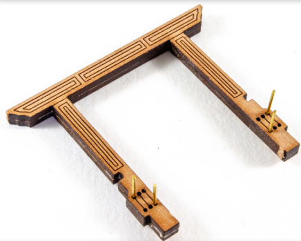
172. Remove the Main Mast Gallews Belaying Rail (150) from the 1mm wood sheet and glue into position as shown. You can also fit photo-etch belaying pins as with the previous bitts and varnish the assembly.
