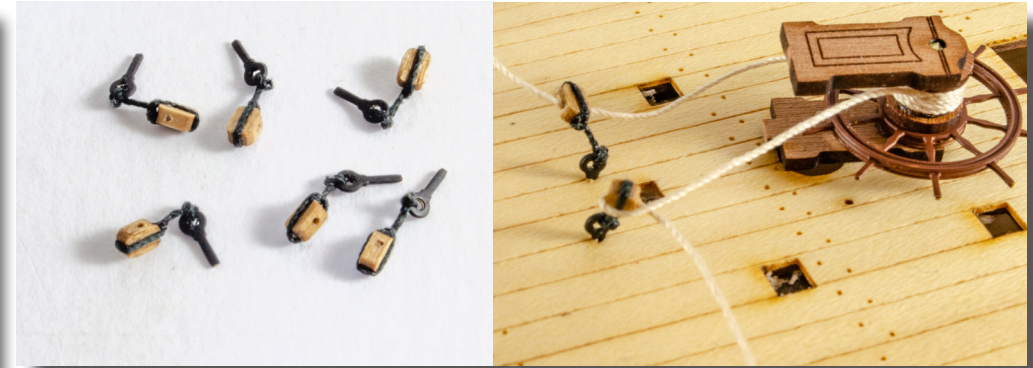
161. Tie six 2mm Single Blocks (F-13) to Standard Eyebolts (PE-90) using 0.25mm black thread (F-25). Fit all blocks into position on the aft deck, as shown on the plan. It's a good idea to spray all the eyebolts in black paint prior to their use (as with other small fittings) and scrape away any paint before gluing in place. Slide the rigging thread on each side of wheel, through the rigging blocks adjacent to wheel. Now glue the wheel unit into position and then rig the blocks as shown here and on plan.
