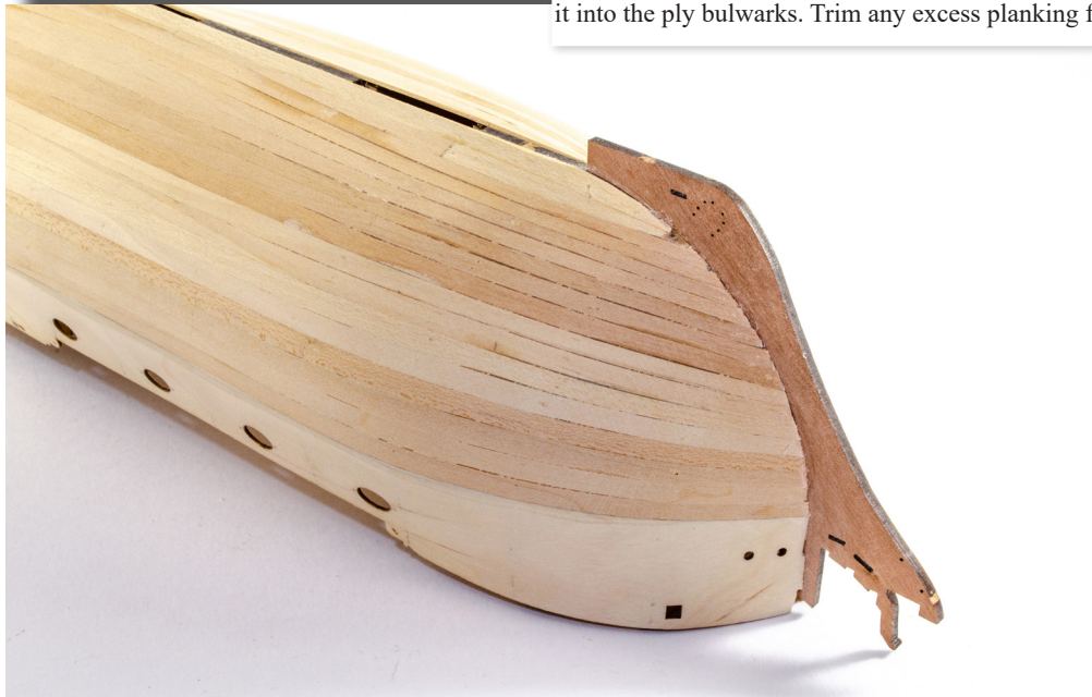
74. Use a sheet of coarse sandpaper (120 grit) and sand smooth the first layer of lime planking, blending it into the ply bulwarks. Trim any excess planking from the stern.
