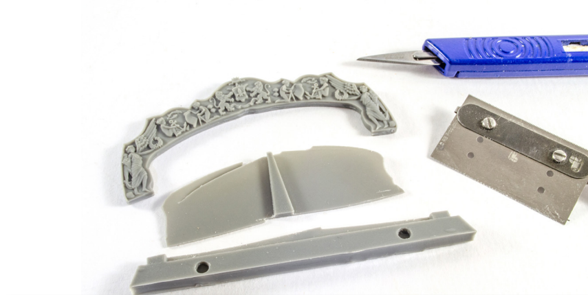
112. Remove the Stern Decoration (F-2) from its casting block using a knife and a razor saw. Clean up any excess resin from the web connection area. This part now needs to be bent to match the curve of the Stern Fascia. This is a very easy task. Dip the part in freshly boiled water for 10-15 seconds, and then remove and immediately lay the part in position. The part will be slightly floppy and mould to the curve of the stern. Leave to cool for a minute, then run under cold water and dry thoroughly.
