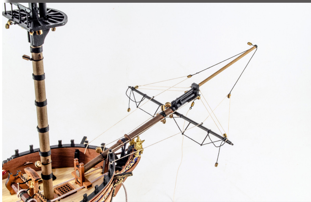
235. Rigging the bowsprit is very easy on this model. First fit the gammoning and then the spritsail boom. Use the rigging illustration on plan sheet #13 to complete this stage.
