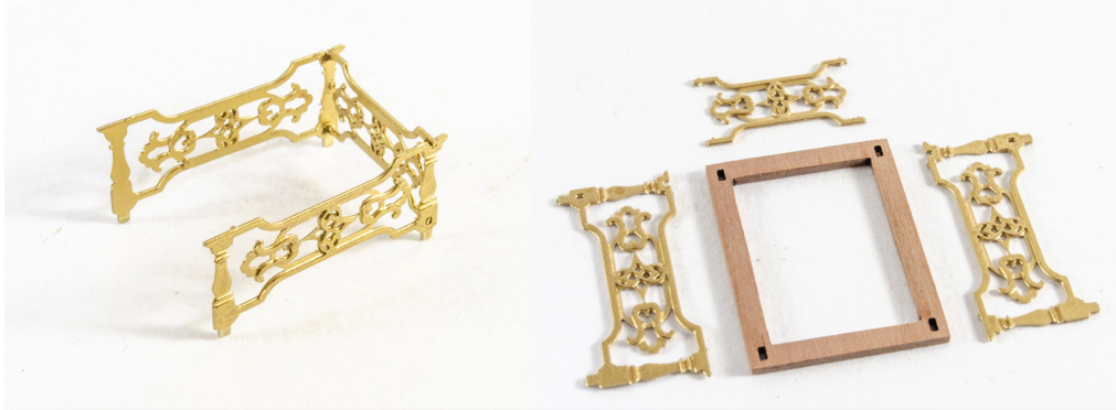
163. Remove the Quarterdeck Companion Rails (PE-97, PE-98, PE-99) from the 0.6mm photo etch sheet, and the Upper Deck Spiral Staircase Coaming (80) from the 1.5mm wood sheet. Using CA, glue the rails together as shown and paint them gold. Also glue the coaming onto the deck as shown. With the parts dry, you can then place the rail onto the coaming and glue into position. At this point, you can also add the Quarterdeck Gunwale Timberheads (99) and paint them black.
