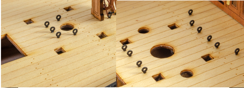
162. Fit Standard Eyebolts (PE-90) to the holes surrounding the mast holes on both decks.
