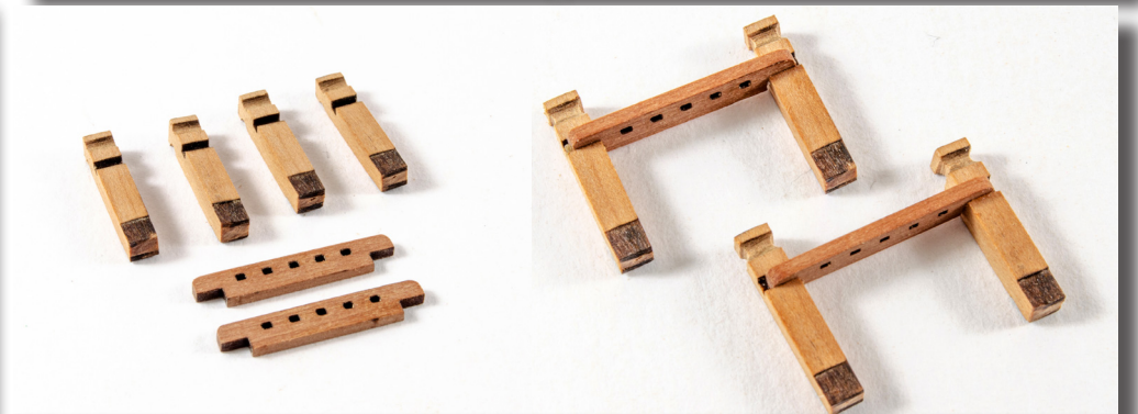
164. Remove the four Mizzen Mast Bitts from the 3mm wood sheet, and the two Mizzen Bitts Belaying Rails (152) from the 1mm wood sheet. Assemble as shown. Note: These look better if you use a small round file to shape the tops of the bitts to make them more 3D. Also remove any char from the visible areas. When complete, add the Belaying Pins (PE-102) as seen and varnish the assembly.
