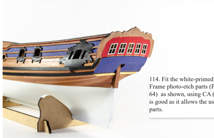
112. Remove the Stern Decoration (F-2) from its casting block using a knife and a razor saw. Clean up any excess resin from the web connection area. This part now needs to be bent to match the curve of the Stern Fascia. This is a very easy task. Dip the part in freshly boiled water for 10-15 seconds, and then remove and immediately lay the part in position. The part will be slightly floppy and mould to the curve of the stern. Leave to cool for a minute, then run under cold water and dry thoroughly.
