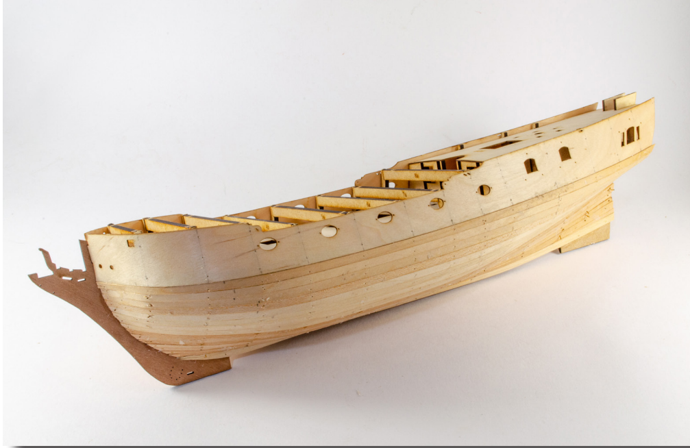
73. Your planked hull should look something like this, as shown in these four photographs. All that matters at this stage is that you have a good surface onto which you will lay the next layer of planks.
