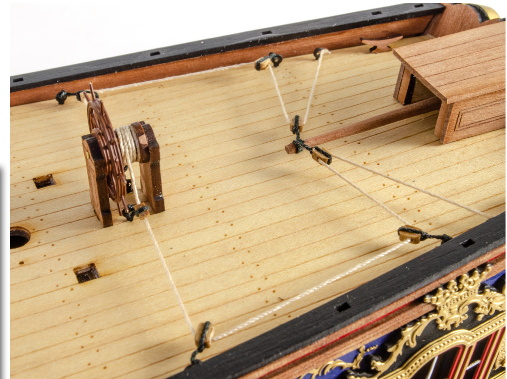
159. Cut around 60cm of 0.25mm natural thread and wrap this around the wheel drum and secure with a little dilute PVA. You should have an equal length of thread loose on either side.
