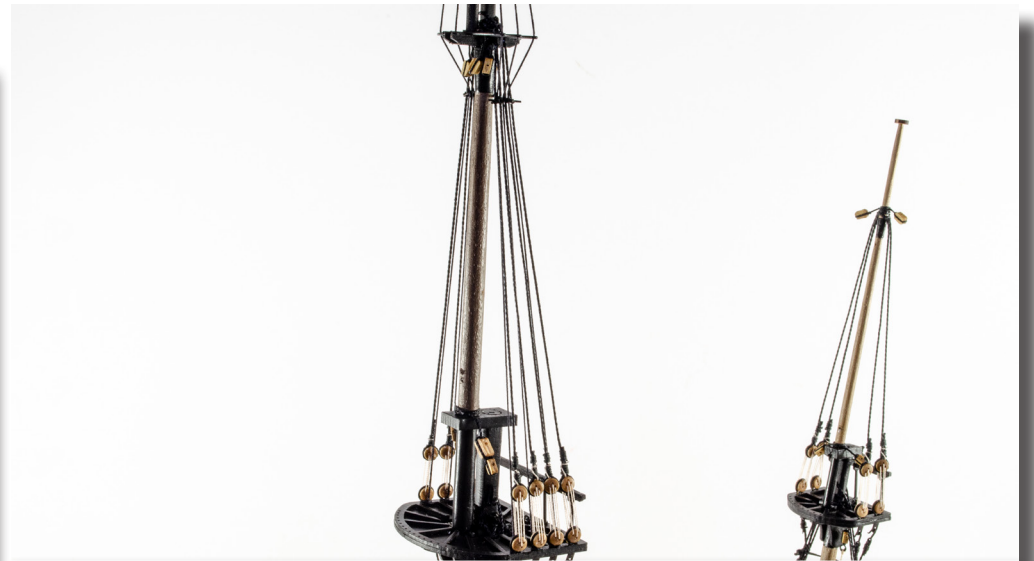
241. Now add the upper shrouds using 0.75mm black thread as shown on plan sheet #11. Add the deadeye lanyards using 0.1mm natural thread and make sure they are reasonably and evenly taught. Be careful not to overtighten them or you'll twist the upper mast.
