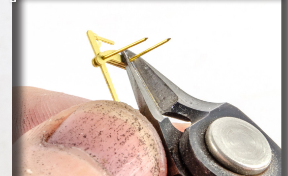
176. Using pins to align, glue a Hand Pump Side Bracket (PE-86) to the Hand Pump Main Body (PE-85). Turn the part over and glue another PE-86 to the opposite side of the pump main body. Glue the pins in position and cut them short as shown.
