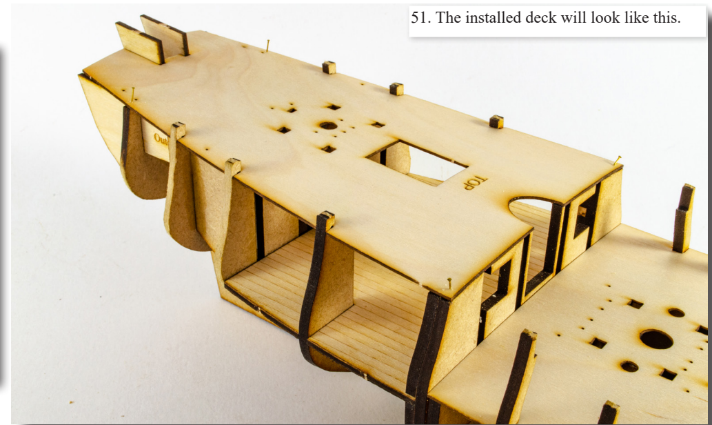
50. We can now fit the Aft Deck in position. Add glue to the top of the various frames and bulkheads, and then flex the plywood deck enough to allow you to fit it into the slots in the bulkhead ears. The deck should fit perfectly in position, sitting flat atop all frames. For extra insurance, you can use brass pins to hold the deck down where it isn't fastened to the bulkhead ears, such as either side of the cabin bulkhead.
