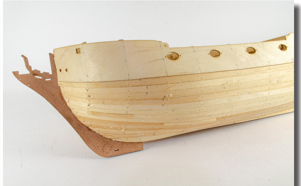
73. Your planked hull should look something like this, as shown in these four photographs. All that matters at this stage is that you have a good surface onto which you will lay the next layer of planks.
