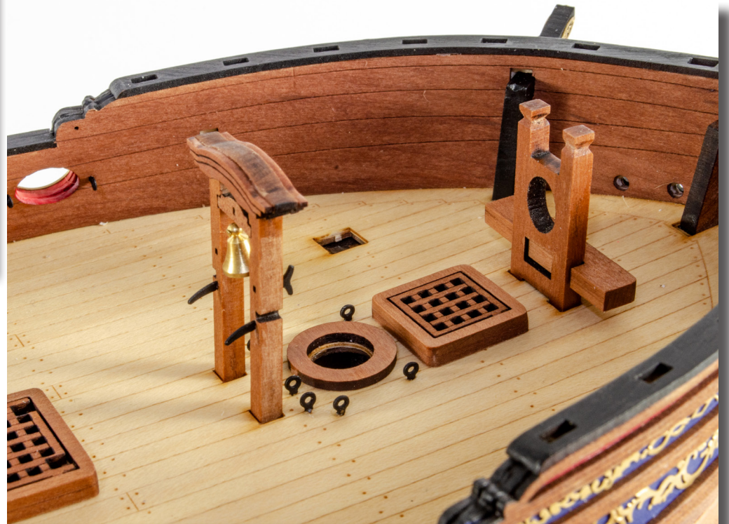
188. Fit the Bell Standard and Bowsprit Bitts as seen in this photo. To be assured the Bell Standard is at the correct height in relation to the winch, you can simply dry fit this for the moment.
