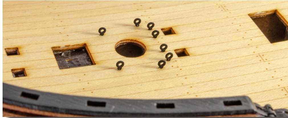
162. Fit Standard Eyebolts (PE-90) to the holes surrounding the mast holes on both decks.
