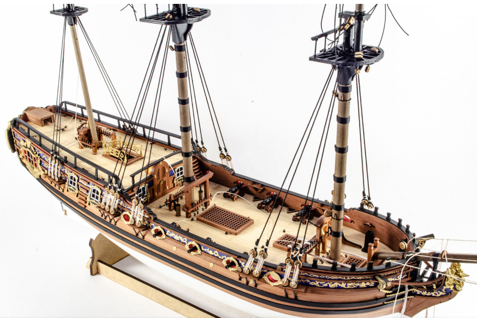
236. The next phase of rigging is to add the shrouds. Use plan sheet #11 for reference with this. The shrouds wrap around the mast sections in sequence and then terminate at the deadeyes. Try to get the deadeyes as level as possible to each other. Tie these to the lower deadeyes as shown on plan sheet #11
