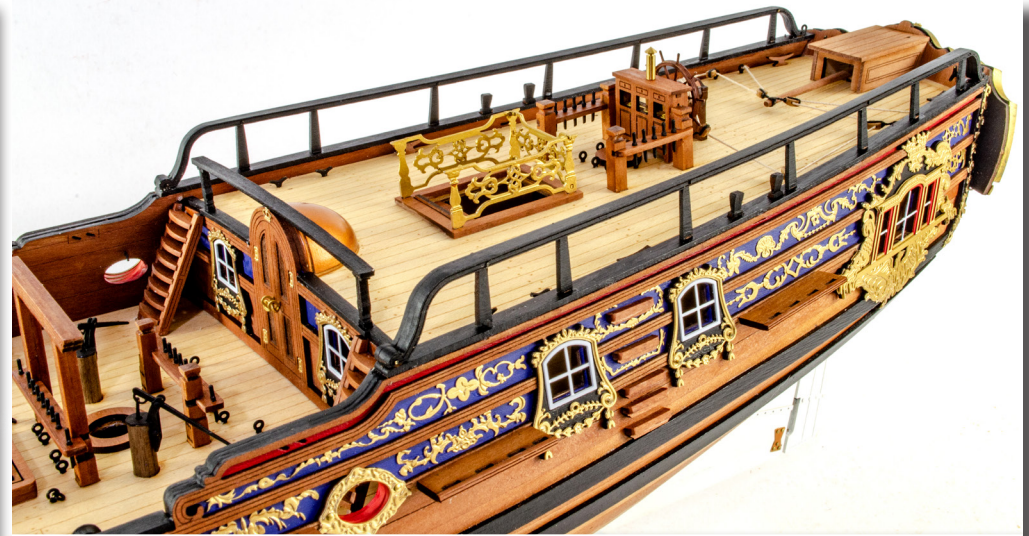
209. Fit the rails to the aft deck gunwales as seen here, making sure that they are also vertical along their length.
