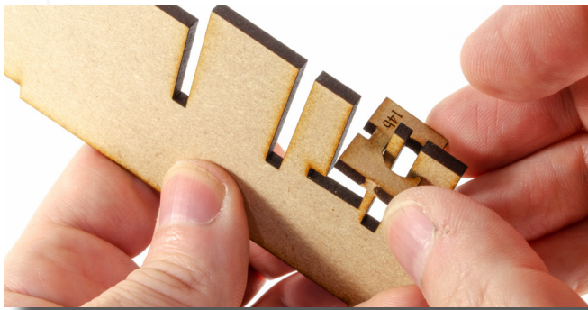
9. Brush a little wood glue around the joint, but not within the mast recess. Note: You will notice that a lot of early MDF construction is glued after the parts are fitted. This is because some modern glues set quickly, and when dealing with multiple slots, it seems a safer way. However, feel free to add glue before fitting parts, if that is what you are more comfortable with.
