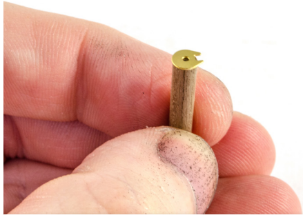
177. Glue the Hand Pump Top Cap onto one end of the dowel. Make sure the PE hole aligns with centre of dowel. Glue the pump assembly into position and then paint black. You can use some metal pigment to give an appearance of iron.
