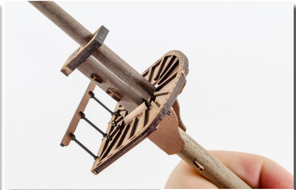
228. Assemble the masts as shown on the plans. These photos will add extra clarity for this stage. Ensure that everything is perfectly straight and in total alignment. Add the various cleats to the masts as shown.
