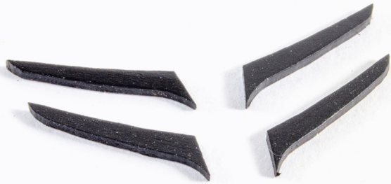
123. Cut the four Bow Brackets (95) from the 1.5mm wood sheet and paint them black.
