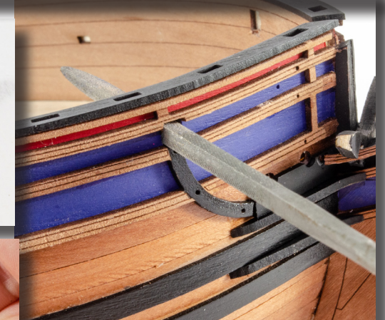
127. Using a flat/square jeweller's file, open up the cathead holes so the cathead will pass through it. You will also need to slightly bevel the underside of the cathead, so it sits flat on the deck. Paint the catheads black and glue them into position as shown here and on plan.
