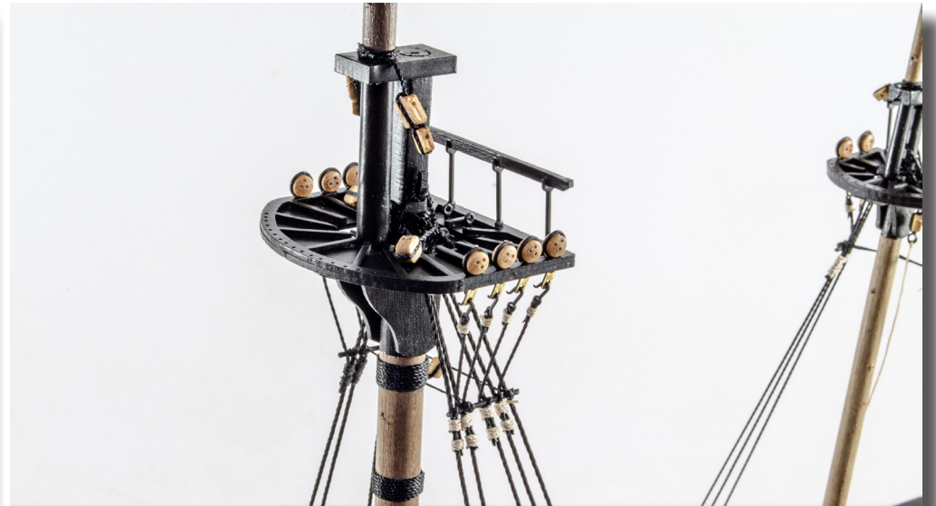
240. After adding the 3mm deadeyes to their 3mm Futtock Stropps (PE-93), slide these into position on the lower mast tops. Now take each futtock shroud line and hook into the stropps, fastening as shown here and on plan sheet #11. Seize with 0.25mm black thread. Again, I have used natural colour thread to illustrate only.
