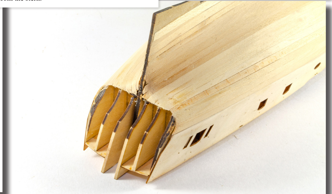
74. Use a sheet of coarse sandpaper (120 grit) and sand smooth the first layer of lime planking, blending it into the ply bulwarks. Trim any excess planking from the stern.
