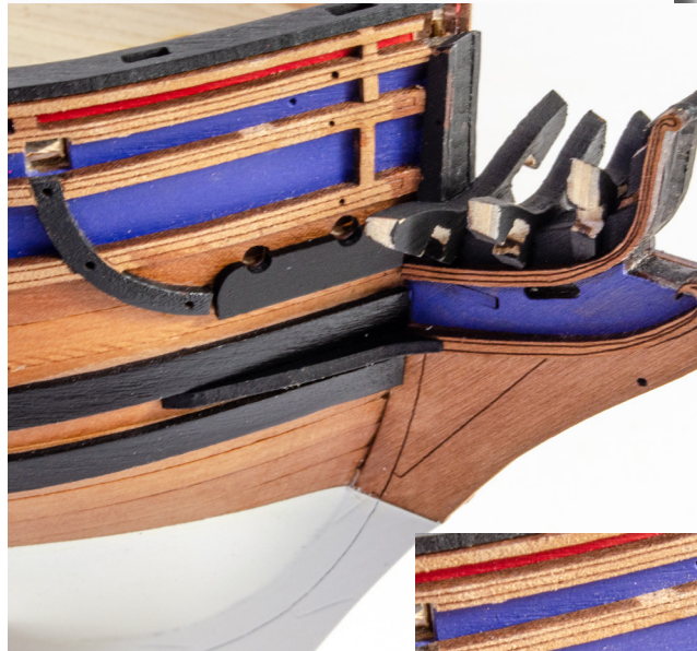
124. Glue two of the bow brackets into position as shown here. Also remove the two Hawse Bolsters from the 1mm wood sheet, paint black, and fit as shown. You may need to trim the inboard edge of these, so the notches are aligned with the hull's hawse holes. Finally, glue the remaining two Bow Brackets into their upper positions, underneath the Hawse Bolsters.
