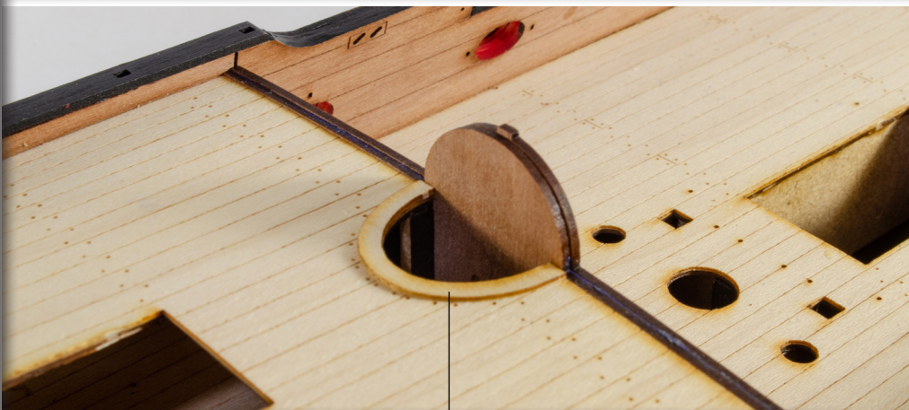
147. Glue the Domed Canopy Base (47) from the 0.8mm veneer, into position as shown.
