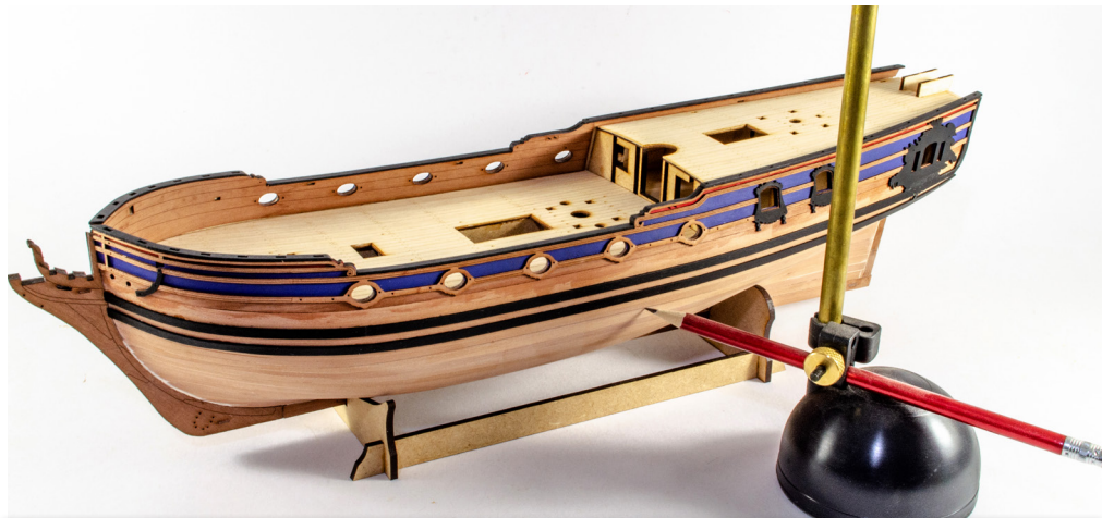
107. A waterline tool is again used to accurately mark the waterline. Use your plan as reference.
