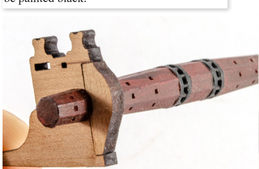
191. Sit the winch drum in the cut-out in the Windlass bitts and glue the Front Pattern into place. Don't glue the actual winch drum. Fit the bitts to both sides of winch drum.
