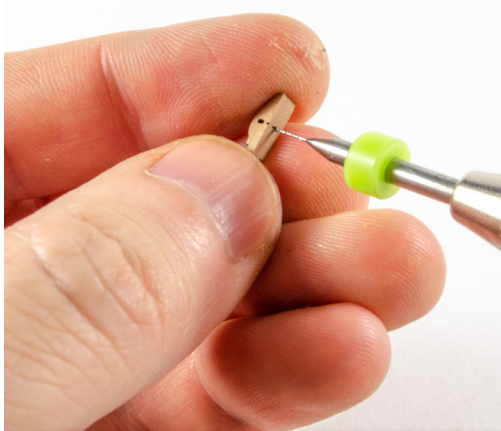
183. Using a 0.5mm drill, make a hole in the bottom of the Head Stock.
