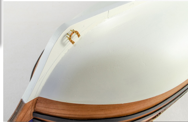
119. Apply a little superglue to the back of one of the Horseshoe Plates and push brass pins through the plate and through the keel so they protrude on the opposite side. Apply a little more superglue to the protruding pins and glue the other Horseshoe Plate in position over the pins. Cut the pins short. Repeat this with the Fish Plate at the stern.
