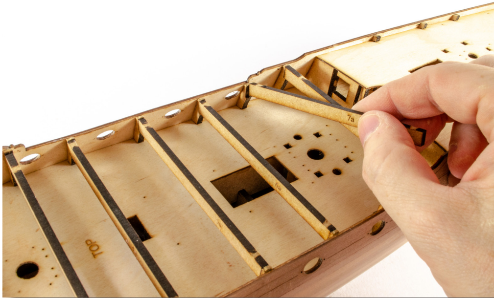
88. The temporary beams can now be twisted and broken off the hull, followed by the MDF bulkhead tabs above the decks. A knife and sandpaper were used to make these flush to the deck. Any glue remnants were also removed from the inner bulwarks.
