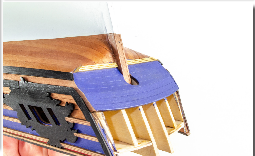
110. After scraping a little blue paint from the lower stern counter, the Wing Transom parts were fitted and trimmed to length.
