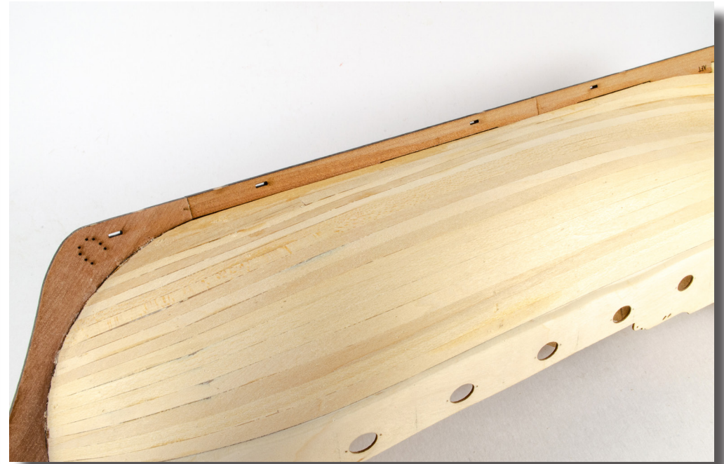
75. Remove the Fore and Aft Keel parts (50, 51) from the 3mm wood sheet, and also the Stern Post (52). Glue the Fore and Aft keel parts into position as shown. They will only fit one way.
