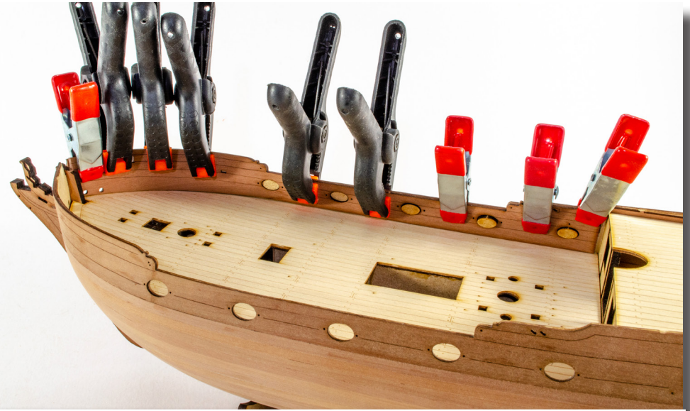
93. Carefully glue the Inner Bulwark Patterns into position and clamp as necessary. We have made these slightly long at the bow side to allow for any hull variations. Make sure that the gun port openings align with the plywood. Use the Oval Side Port Locator Plugs from the 6mm MDF (225) so assist you. These will be removed once the bulwarks are set.
