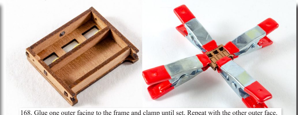
168. Glue one outer facing to the frame and clamp until set. Repeat with the other outer face.
