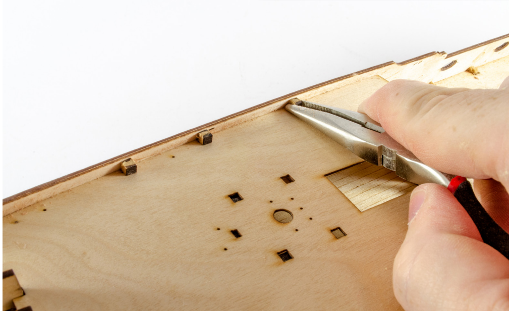
88. The temporary beams can now be twisted and broken off the hull, followed by the MDF bulkhead tabs above the decks. A knife and sandpaper were used to make these flush to the deck. Any glue remnants were also removed from the inner bulwarks.
